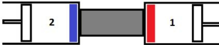
Figure 1.1. Alpha Stirling machine, where 1 is the expansion space with the cold heat exchanger, 2 is the compression space with the warm heat exchanger, and the connecting portion is the regenerator.
