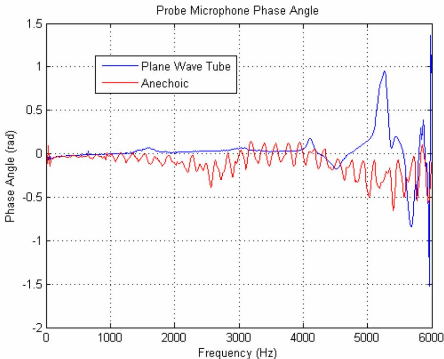
**Figure 5: Anechoic vs. Plane Wave Tube Phase Angles for Probe Microphones**
