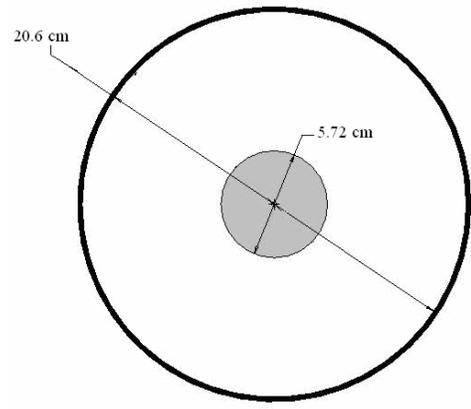
**Figure 7: Duct Cross Section with Center Body**
