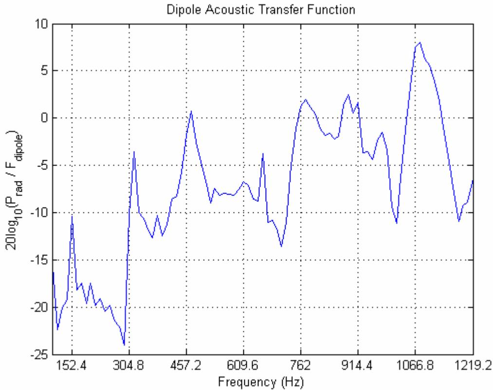
**Figure 10: “Organ Pipe” Duct Modes at Lower Frequencies**
