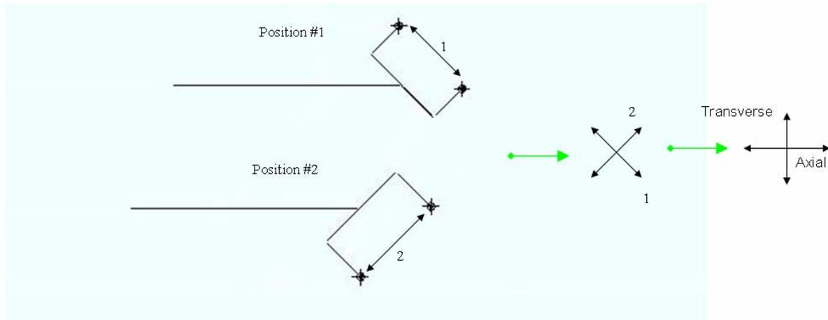
**Figure 4: Obtaining Axial and Transverse Dipole acoustic transfer functions**
