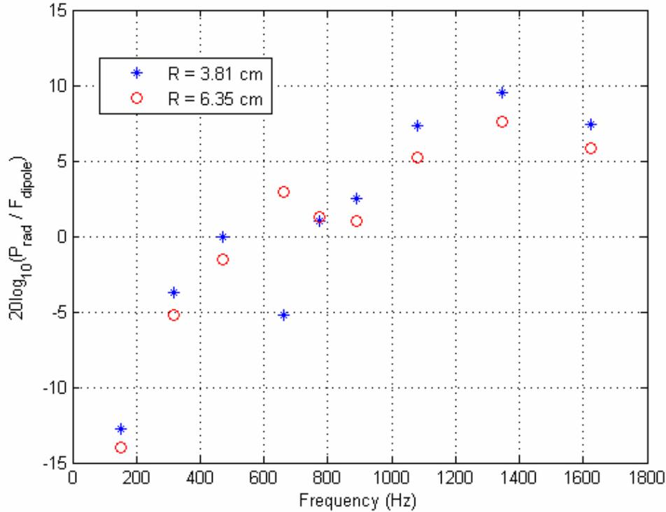
**Figure 13: Magnitude of the Transfer Function at the first nine duct modes for two different radial positions**
