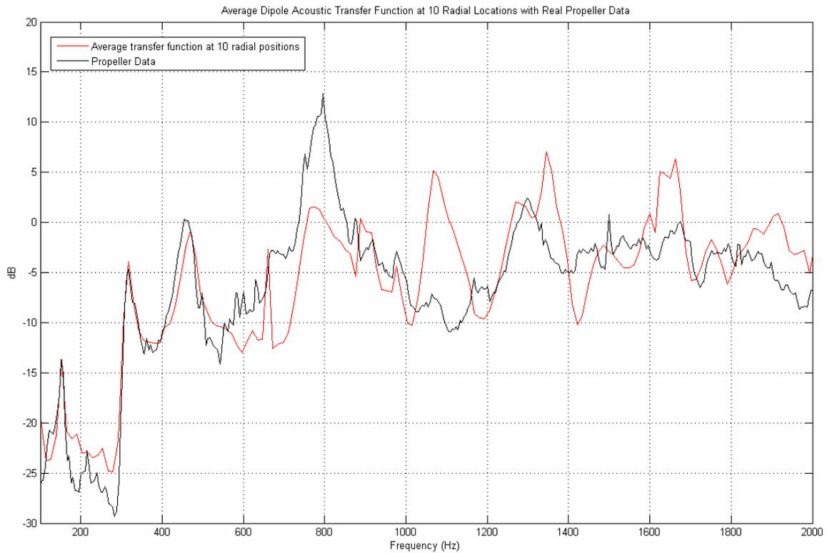
**Figure 15: Comparison of Average Transfer Function with Results Obtained Using Propeller**
