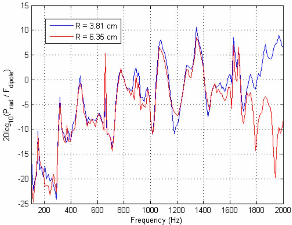
**Figure 12: Radial Dependence of Transfer Function**
