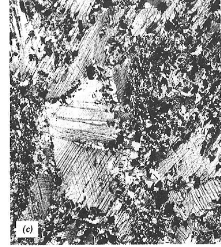
partial recrystallization (4 s at 580°C)
