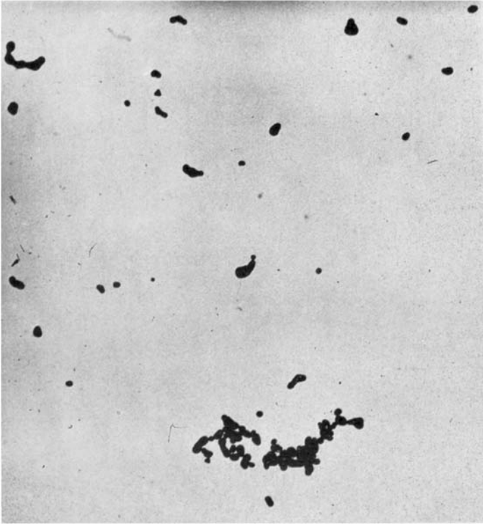
FIG. 1.—Electron micrograph of a gold sol reduced with carbon monoxide, magnification of 50,000 diameters.
