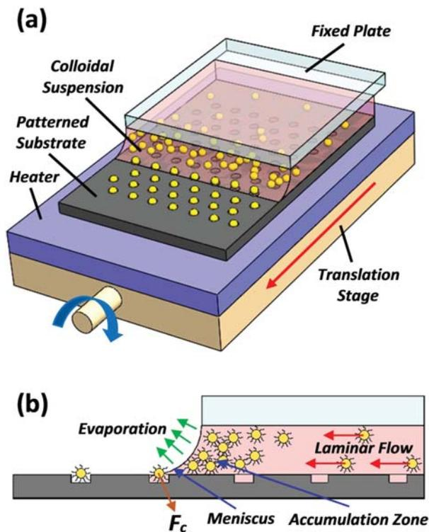
**Figure 1.** Schematics showing (a) the instrumentation used in the capillary assembly of colloidal nanostructures on lithographically patterned surfaces and (b) the essential mechanistic features of the assembly process that include (i) the laminar flow of nanostructures to the accumulation zone, (ii) a receding meniscus caused by evaporation and substrate translation, and (iii) nanostructures being driven into recessed features by the downward component of the capillary force ( $F_c$ ).
