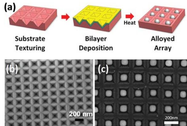
**Figure 7.** (a) Schematic of the templated dewetting process used to generate periodic arrays of CoPt nanoparticles using a textured substrate. SEM images of a (b) textured substrate and (c) the array of CoPt nanoparticles formed after the dewetting of a Co/Pt bilayer. (7b reproduced with permission from [107]. Copyright 2009 Wiley.) (7c reproduced with permission from [76]. Copyright 2013 Wiley.)
