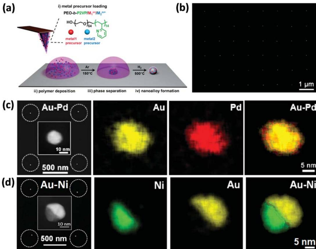
**Figure 9.** (a) Schematic of the scanning probe block copolymer lithography (SPBCL) process used to fabricate arrays of alloyed nanostructures. (b) SEM image of an array of AuPd nanoparticles. High-angle annular dark-field scanning transmission electron microscopy (HAADF-STEM) images and elemental mapping for (c) alloyed AuPd and (d) phase-segregated Au/Ni nanostructures. (Reproduced with permission from [123]. Copyright 2015 American Chemical Society.)
