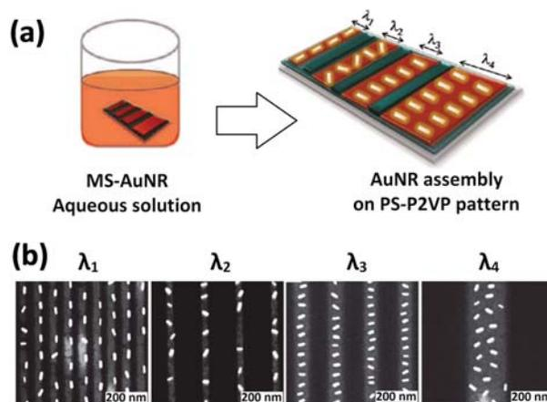
**Figure 5.** (a) Schematic showing a chemically nanopatterned surface with areas promoting (red) and inhibiting (green) nanorod attachment. (b) SEM images showing the nanorod patterns obtained as the width of the patterned strip ( $\lambda$ ) is varied. (Reproduced with permission from [42]. Copyright 2012 American Chemical Society.)
