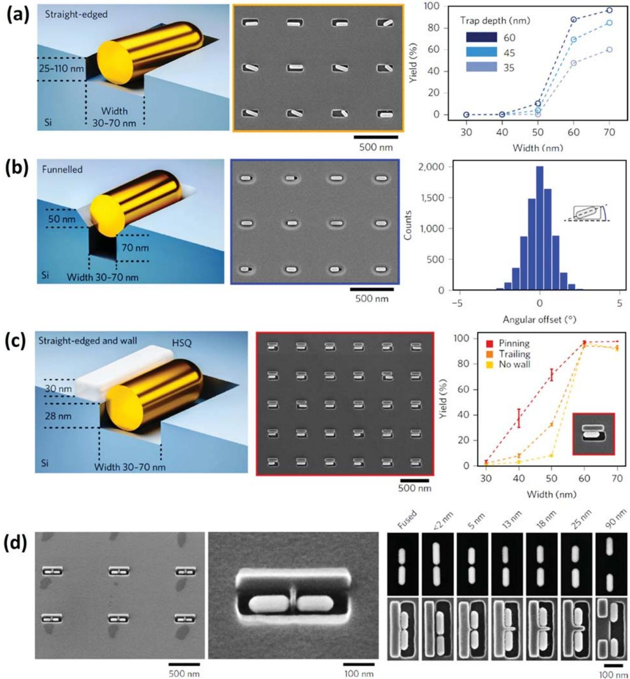
**Figure 3.** Schematics, SEM images, and a statistical analysis of the trapping performance for traps having (a) straight-edged sidewalls, (b) tapered sidewalls, and (c) an auxiliary sidewall. (d) SEM images demonstrating the nanoscale control achievable in the spacing between two end-to-end aligned nanorods positioned using the biasing capability of auxiliary sidewalls. (Reproduced with permission from [52]. Copyright 2017 Macmillan Publishers Ltd.)
