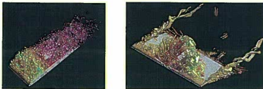
Examples of dynamic stall over 2D and 3D wing configurations
