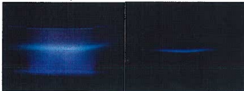
Plasma (24 kHz, 15 W) assisted methane flame
