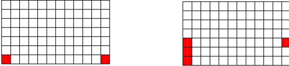
Figure 26: Two representations of the support location on the wing box for the normal HCA code (left) and the support optimization HCA code (right). Note that only the outside region is eligible for support placement.
