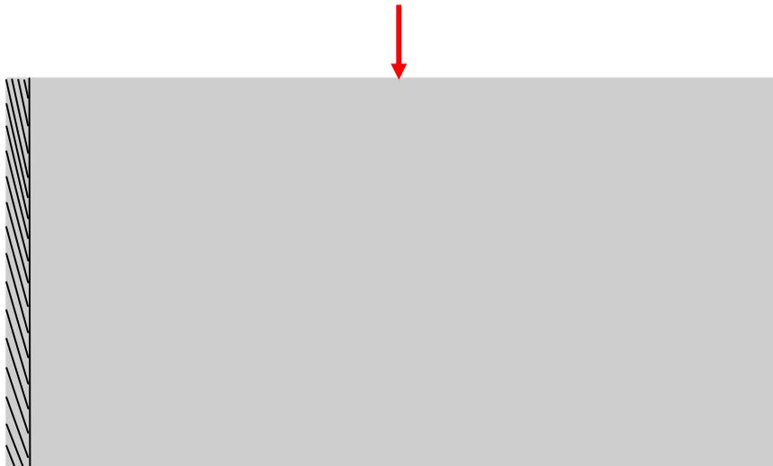
Figure 12: 20 X 40 rectangular design domain with load at top center and optimization region on left side. The initial mass fraction was 0.2.
